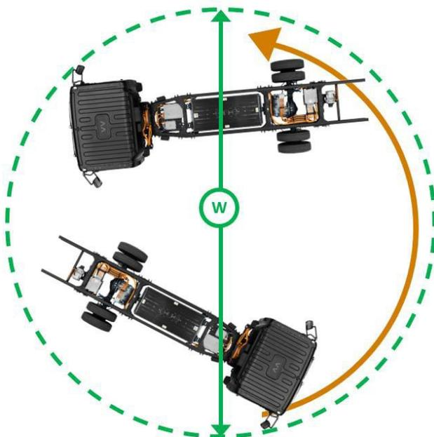
W = Minimum turning diameter wall to wall
