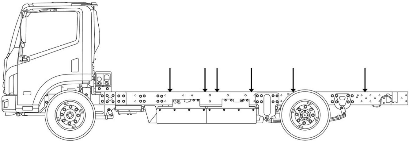
When using U-Bolts to attach a body structure, the points above are the only recommended positions for attachment.
